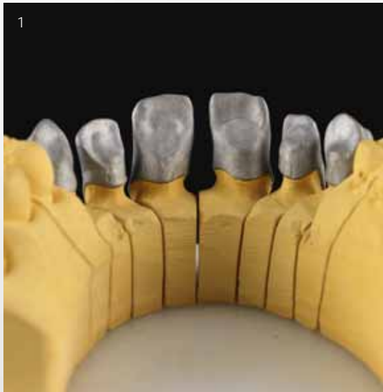
Fig. 1 and 2 Using the new processing technology crown and bridge frameworks can be milled in the usual way from Ceramill Sintron in the green body state. The frameworks achieve their usual material properties in a subsequent sinter process under shielding gas.
